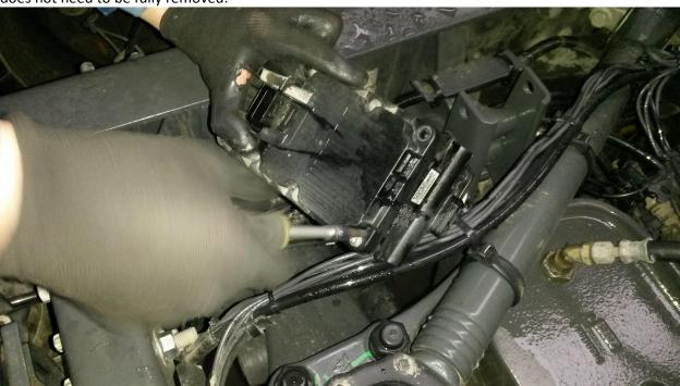
3 step. Solder cables to the connector pin. Take off the resistance indicated by the arrow and in that place we solder white wire. Pay attention to the white wire soldered area!!!!!
