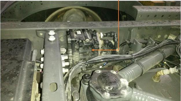
2 step. Unscrew the valve from the frame, disconnect the connector and remove the cover. The valve does not need to be fully removed.
