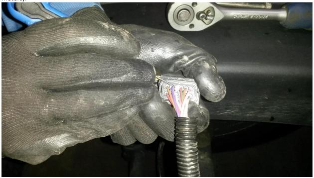
6 step. The cab connect the switch and LED:
